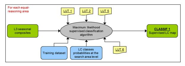
Figure 3-8: Activity diagram illustrating the Gaussian Maximum Likelihood supervised classification algorithm developed in the CCI-LC project
