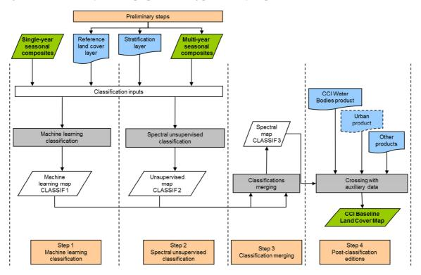
Figure 3-1: Schematic representation of the classification process developed to generate a baseline global LC map over the period 2003-2012 using the entire archives of Envisat MERIS data
