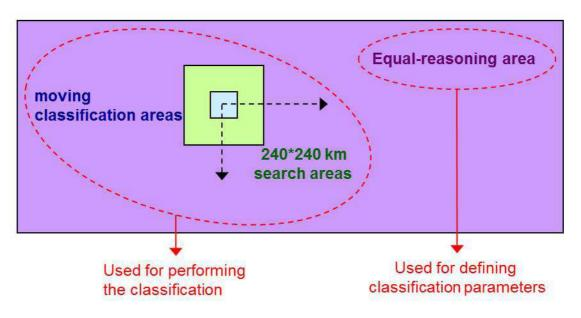
Figure 3-5: Illustration of the tree spatial units (equal-reasoning, classification and search areas) of the developed locally-adjusted supervised classification procedure
