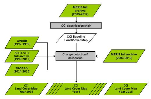
Figure 2-1: Schematic representation of the CCI-LC classification chain made of 2 main processes to generate global annual LC maps using the entire archives of Envisat MERIS, AVHRR time series between 1992 to 1999, SPOT-VGT time series between 1999 and 2013 and PROBA-V data for 2014 and 2015.
