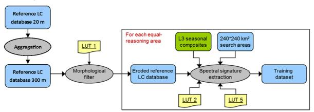
Figure 3-6: Activity diagram illustrating the training dataset preparation: (1) the reference land cover database is aggregated to 300 m, (2) the reference land cover database is eroded and (3) spectral signatures are extracted or each eroded class
