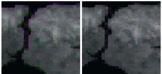
When looking at the coastline in the left figure a RR shift is clearly visible. The order of magnitude of this shift is about 1RR pixel, i.e. about 4 FSG. After applying AMORGOS 4.0 the excellent relative geolocation accuracy of RRG and FSG is observed.
